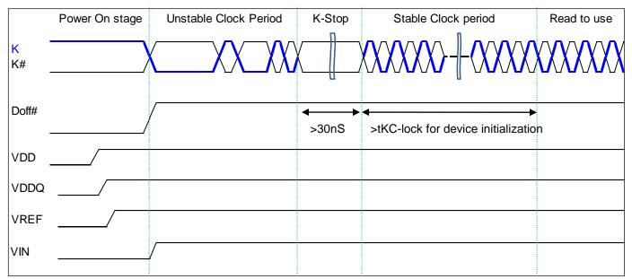
Note) All inputs including clocks must be either logically High or Low during Power On stage. Timing above shows only one of cases.
