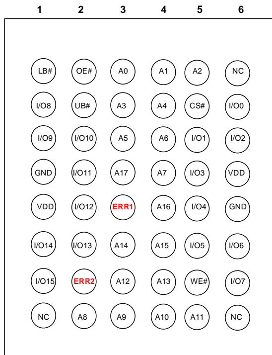
**48-Pin mini BGA (6mm x 8mm),2CS, ERR1/ERR2**
