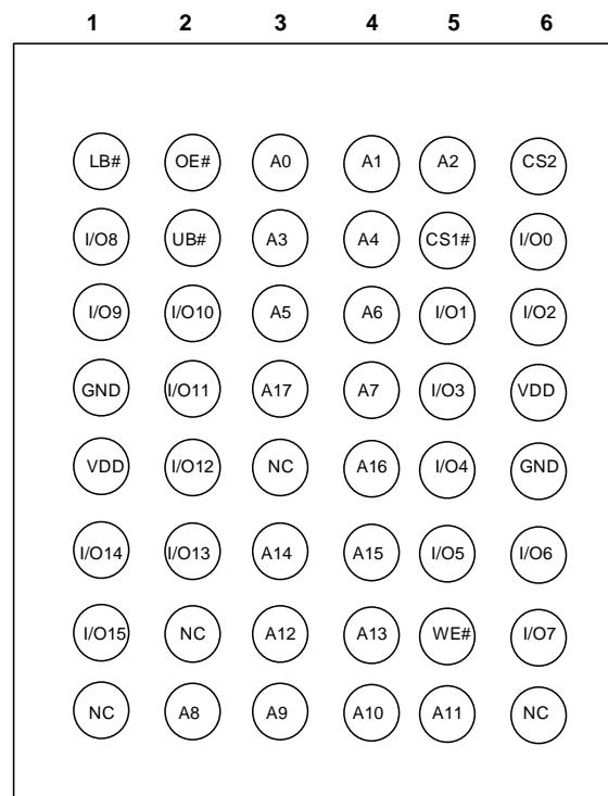
**48-Pin mini BGA (6mm x 8mm),1CS, ERR1/ERR2**
