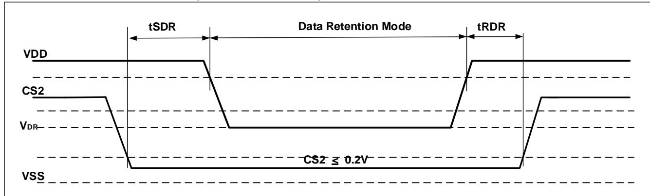
DATA RETENTION WAVEFORM (UB# AND LB# CONTROLLED)
