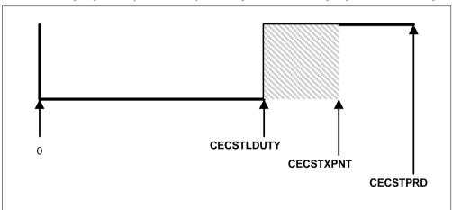
The following registers are used for START detection.
