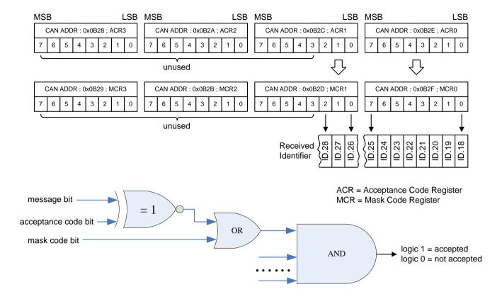
Standard frame: if a standard format frame message is received, the completely identifier are used for acceptance filtering. For a successful reception of a frame, all single bit comparisons have to signal acceptance. Note that ACR3, MCR3, ACR2, MCR2 and the 5 most significant bits of ACR1 and MCR1 are not used. In order to be compatible with future products, these unused bits in Mask Code registers should be programmed to be 'don't care' by setting these bits to logic 1.
