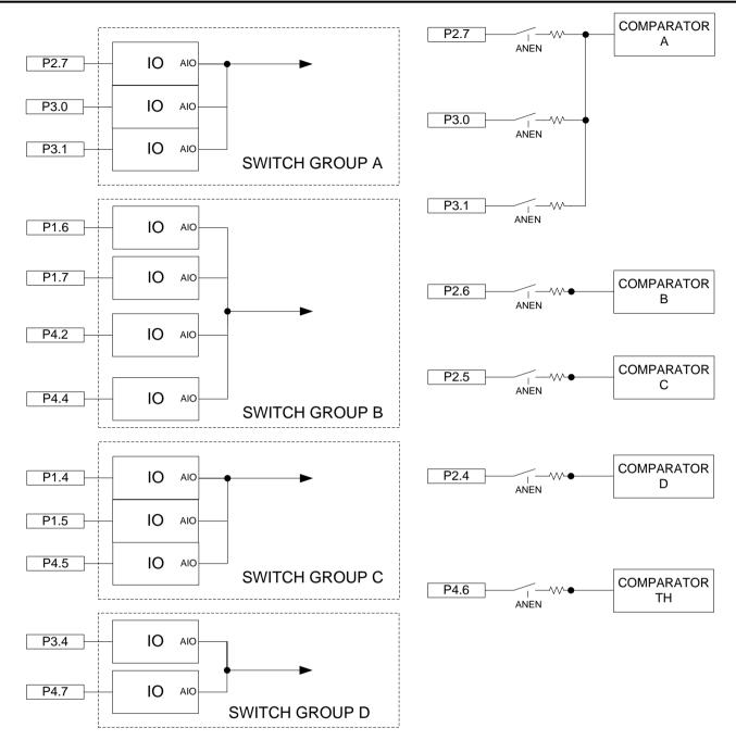
The right is the equivalent circuit. The resistor is the equivalent resistor of the analog switch which is typically less than 1K Ohm. Using ANEN control, analog multiplexer can be achieved. The input/output range of the analog signal is limited to 0 – VDD.
