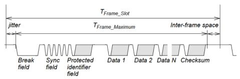
LIN bus protocol is based on frame. Each frame is partitioned into several parts as shown above. For master to initiate a frame, the software follows the following procedure.
