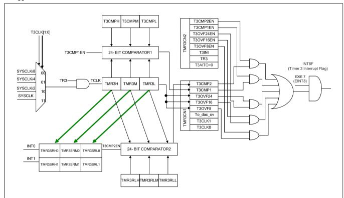
When T3AUTO is 1, T3 operates at AUTO-RELOAD mode. TMR3[23-0] counter increments and overflows from 0xFFFFFF then reload from the register TMR3RL[23-0]. TheAUTO-RELOAD operation is shown in the following diagram.
