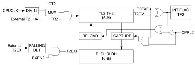
The block diagram of the Timer 2 operating in Baud Rate Generator is shown in the following diagram.
