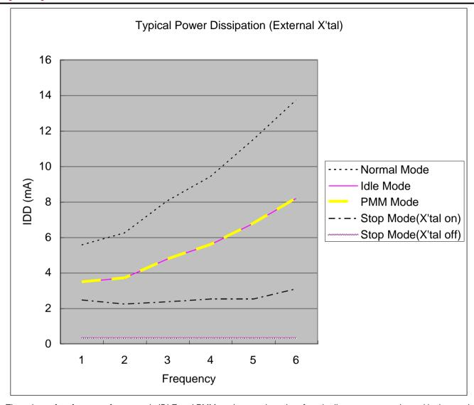
The values of performance frequency in IDLE and PMM modes are close therefore the lines appear overlapped in the graph.
