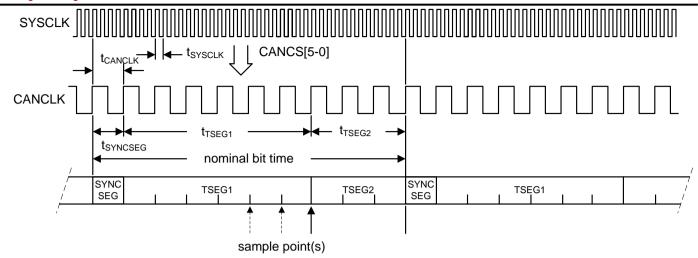
CAN baud rate is thus can be calculated as CANCLK/((TSEG2[2-0]+1)+(TSEG1[3-0]+1)+1). Or in terms of SYSCLK, SYSCLK/2/(CANCS[5-0]+1)/{(TSEG2[2-0]+1)+(TSEG1[3-0]+1)+1}. Also note, with re-synchronization, a delay compensation segment is inserted between SYNC SEG and TSEG1. The maximum length of delay compensation segment is limited by SJW[1-0].
