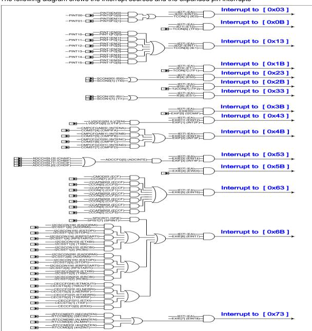
The interrupt related registers are listed in the following. Each interrupt can individually enabled or disabled by setting or clearing corresponding bit in IE and EXIE and integrated peripherals' control registers.
