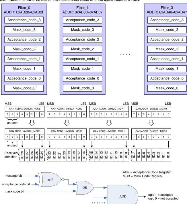
Extended frame: if an extended format frame is received, the complete identifier including the RTR bit is used for acceptance filtering. For a successful reception of a message, all single bit comparisons have to signal acceptance. It should be noted that the 3 most significant bits of ACR3 and MCR3 are not used. In order to be compatible with future products these bit should be 'don't care' by setting MCR3.7, MCR3.6 and MCR3.5 to logic 1.
