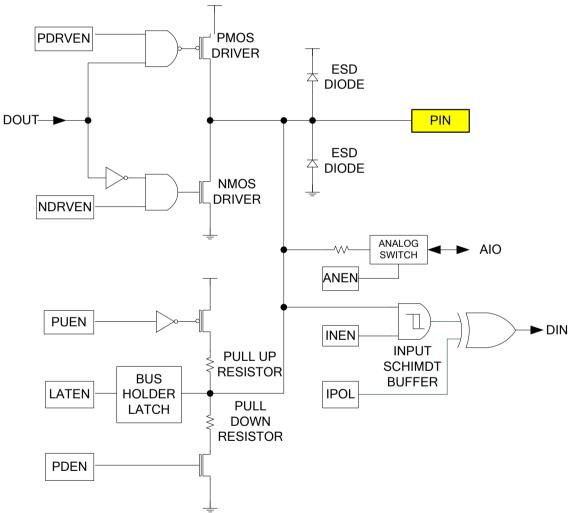
Please note for those pins denoted as OD (Open Drain), P1.3 (SCL), P1.2 (SDA), P4.0 (CEC), P4.1 (SDA2), P4.3 (SCL2), the upper side ESD diode, PMOS Driver, and Analog Switch are removed. This allows the external pullup of the OD pins to be connected up to 12V.
