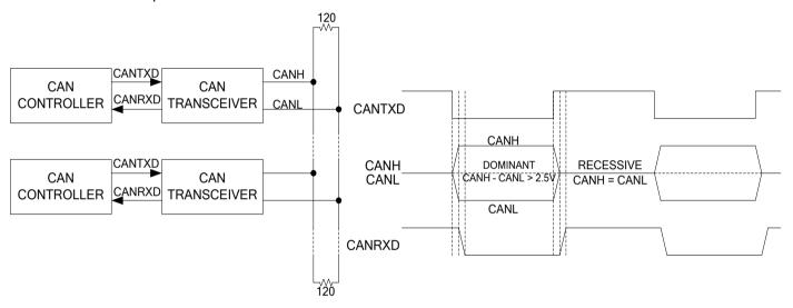
The CAN protocol is a modified version of Carrier Sense Multiple Access/Collision Avoidance (CSMA/CA) similar to Ethernet. If two nodes are trying to send at the same time, instead of collision avoidance, the ID field of message will resolve itself which allows the higher priority message to continue and lower priority message been postponed. The typical standard CAN frame format and extended format are shown in the following.
