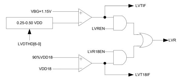
An enabled LVD circuit consumes about 100uA to 400uA depending on its VDD level. The LVDTHD[6-0] sets the compare threshold from 0.25VDD to 0.50VDD against the internal band-gap reference voltage of 1.15V. The detection threshold can be represented in the following equation when LVDTHV is the detection voltage.
