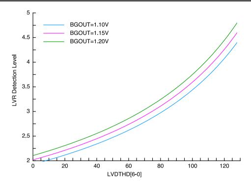
For very precise detection level, the manufacturing process stores the LVDTHD value for detection of 4.0V and 3.0V in IFB. The user program can then use these two values and obtain a real average BGOUT value using the above formula. Then use the real BGOUT value to obtain the specific LVDTHD value for an arbitrary detection level.
