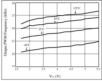
Figure 9 Output PWM Frequency vs. V<sub>CC</sub>
