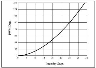
Figure 7 Gamma Correction (32 Steps)
