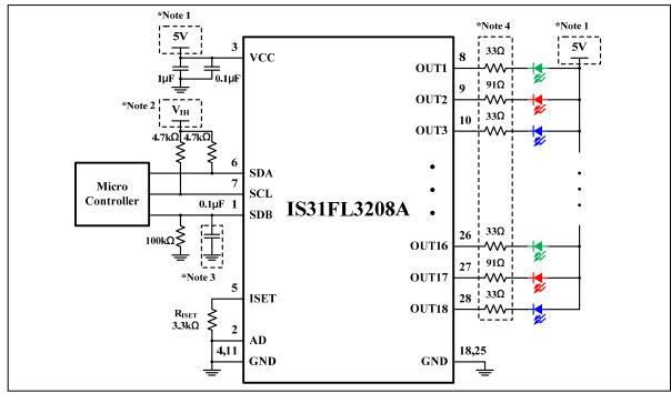
Figure 2 Typical Application Circuit (V<sub>CC</sub>= 5V)
