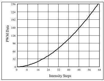
Figure 8 Gamma Correction (64 Steps)
