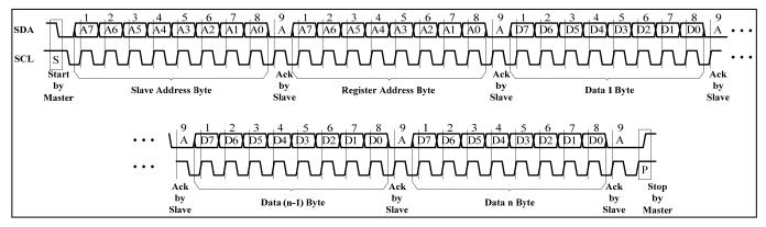
Figure 6 Writing to IS31FL3208A (Automatic Address Increment)
