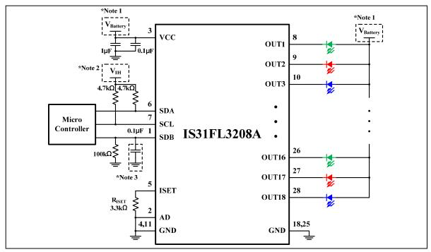
Figure 1 Typical Application Circuit (V<sub>CC</sub>= Battery)
