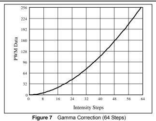
Note, the data of 32 gamma steps is the standard value and the data of 64 gamma steps is the recommended value.
