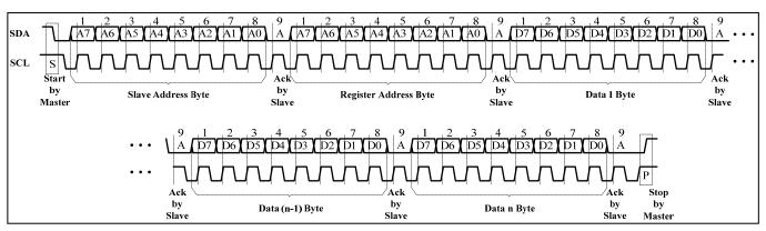
Figure 5 Writing to IS31FL3218 (Automatic Address Increment)
