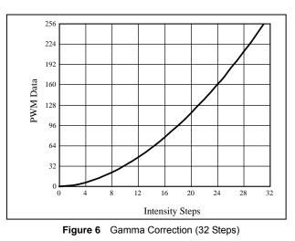
Choosing more gamma steps provides for a more continuous looking breathing effect. This is useful for very long breathing cycles. The recommended configuration is defined by the breath cycle T. When T=1s, choose 32 gamma steps, when T=2s, choose 64 gamma steps. The user must decide the final number of gamma steps not only by the LED itself, but also based on the visual performance of the finished product.
