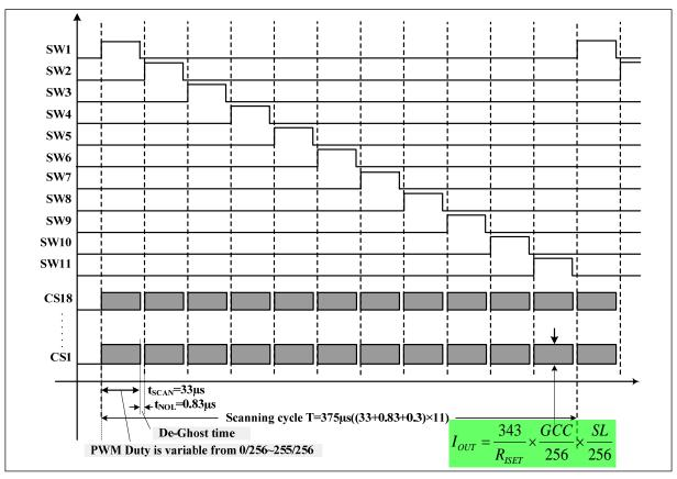
Figure 12 Scanning Timing
