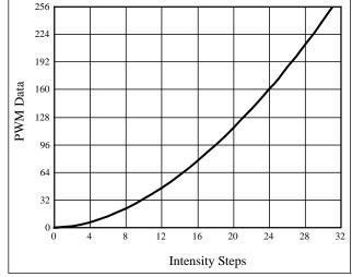
Figure 13 Gamma Correction (32 Steps)
