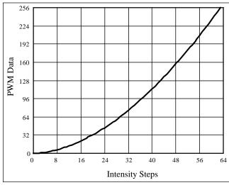
Figure 14 Gamma Correction (64 Steps)
