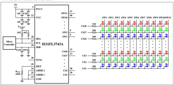
Figure 1 Typical Application Circuit: 66 RGBs
