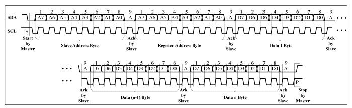
Figure 7 I2C Writing to IS31FL3743A (Automatic Address Increment)
