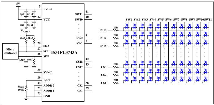
Figure 2 Typical Application Circuit: 198 Mono Color LEDs
