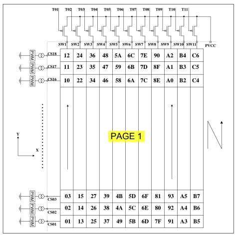
Figure 10 Scaling Register
