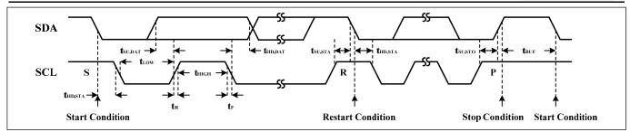
Figure 4 I2C Interface Timing
