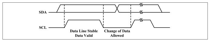
Figure 5 I2C Bit Transfer
