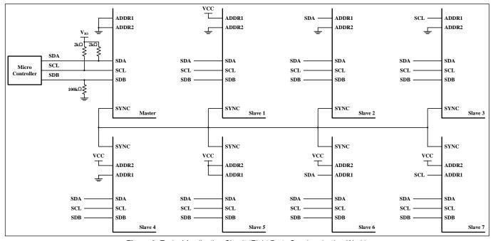
Figure 3 Typical Application Circuit (Eight Parts Synchronization-Work)
