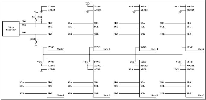
Figure 2 Typical Application Circuit (Eight Parts Synchronization-Work)
