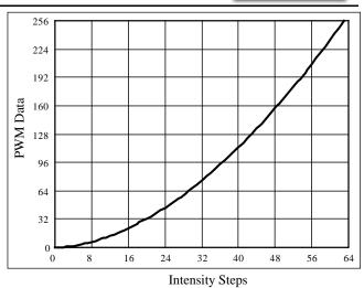
Figure 14 Gamma Correction (64 Steps)
