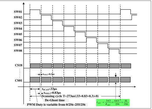
Figure 12 Scanning Timing
