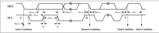
Figure 4 I2C Interface Timing
