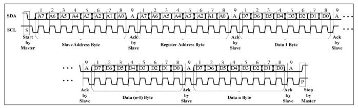
Figure 7 I2C Writing to IS31FL3745 (Automatic Address Increment)
