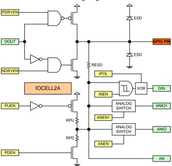
IOCELL2A is IOCELL with two analog multiplexer switches, ANIO and ANIO1. The control of IOCELL2A uses IOCFG's ANEN1 to replace LATEN.
