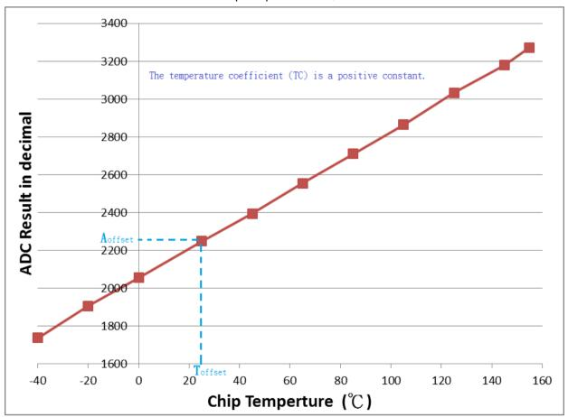
In IS32CS8973, the temperature coefficient (TC) is a positive constant. This calibration value can be found in the Flash Information Block (IFB) address 0x2D. The byte contains the calibrated temperature coefficient for 1°C in LSB of ADC. This is a binary number in 4:4 formats, i.e. the radix point is between bit 4 and bit 3. For example, 0b0111.1100 refers to 7.75 LSB. If calibration of temperature sensor is not done, then this byte would be written as 0x00.
