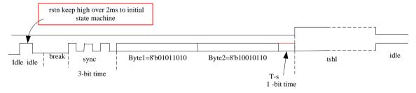
The sequence is initiated for RSTN=0 > 4msec (BREAK field), then followed by three SYNC bit, and two bytes sequence and a T-S bit. RSTN then must return to 0 to maintain the test mode. If the sequence is not exactly matched, a BREAK field must be inserted to start over the sequence. The hardware block diagram is shown in the following and key parameters are also illustrated.
