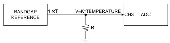
The current is applied to an on-chip low temperature coefficient resistor and develops to a voltage that is in terms proportional to the temperature. The voltage can be written in as an equation of V = K \* Temperature, where K is a constant. The following graph shows the temperature sensor curve with the ADC Result. The vertical axis is the ADC Result in decimal and the horizontal axis is the chip temperature in  $^{\circ}\mathbb{C}$ .
