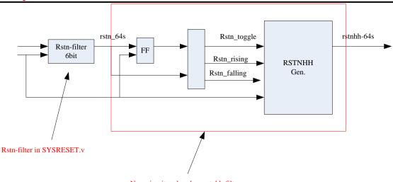
New circuit and replace rstnhh-filter in SYSRESET.v
