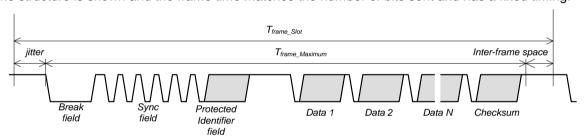
LIN bus protocol is based on frame. Each frame is partitioned into several parts as shown above. For master to initiate a frame, the software follows the following procedure.
