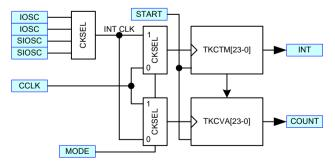
When MODE=0 (MODE0), the counter uses internal clock and timer uses sensing clock. This typically is used when the capacitance oscillation is slower. When MODE=1 (MODE1), the clock relationship is reversed and this is typically used when sensing oscillation is faster. Typical waveforms are shown in the following timing diagram.
