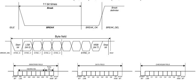
A LIN frame structure is shown and the frame time matches the number of bits sent and has a fixed timing.
