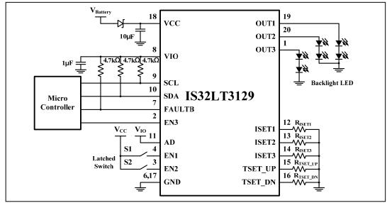
Figure 2 Typical Application Circuit with Latched Switch
