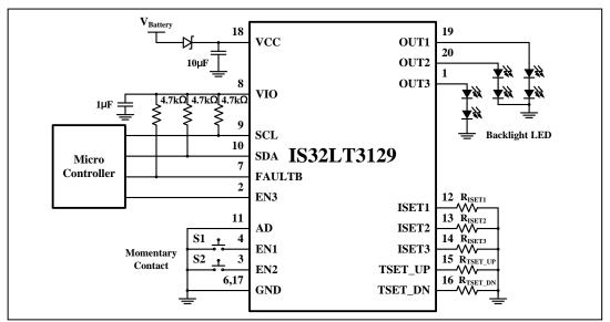
Figure 1 Typical Application Circuit with Momentary Contact Switch
