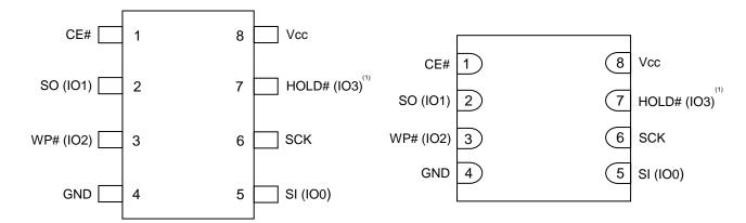
8-pin SOIC 208mil 8-pin VSOP 208mil
