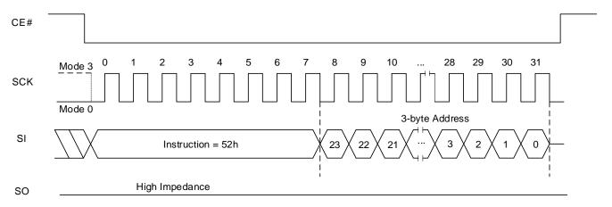
Figure 8.19 Block Erase (32K) QPI Sequence
