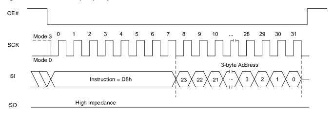
Figure 8.17 Block Erase (64K) QPI Sequence
