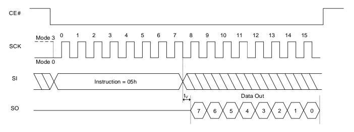
Figure 8.27 Read Status Register QPI Sequence
