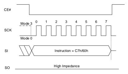
Figure 8.21 Chip Erase QPI Sequence
