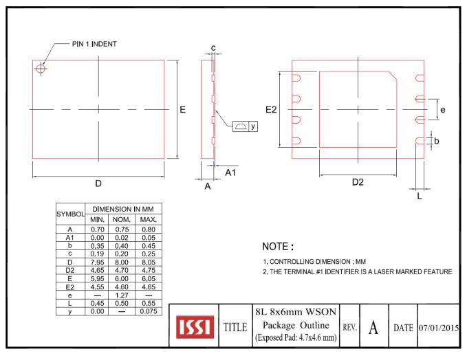
Note: All dimensions are in millimeters. Lead co-planarity is 0.08mm.
