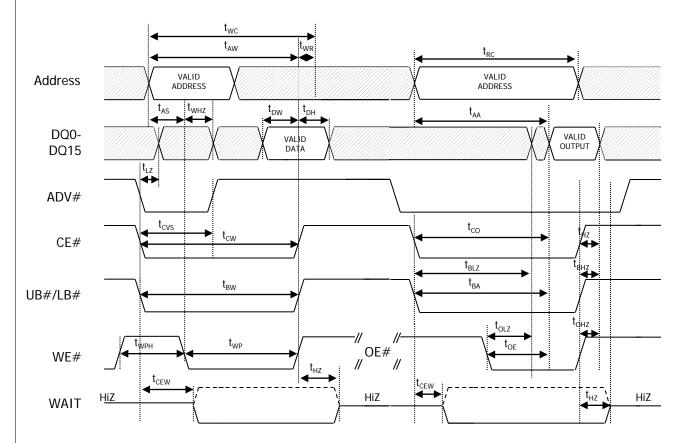
1. When configured for synchronous mode (BCR[15] = 0), CE# must remain HIGH for at least 5ns (tCPH) to schedule the appropriate refresh interval. Otherwise, tCPH is only required after CE#-controlled WRITEs.
