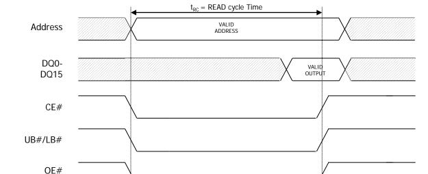
Figure 4. Asynchronous Read Access Timing (ADV# LOW)
