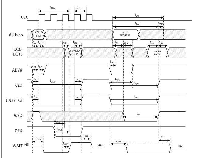
Figure 48: Burst READ Followed by Asynchronous WRITE Using ADV#
