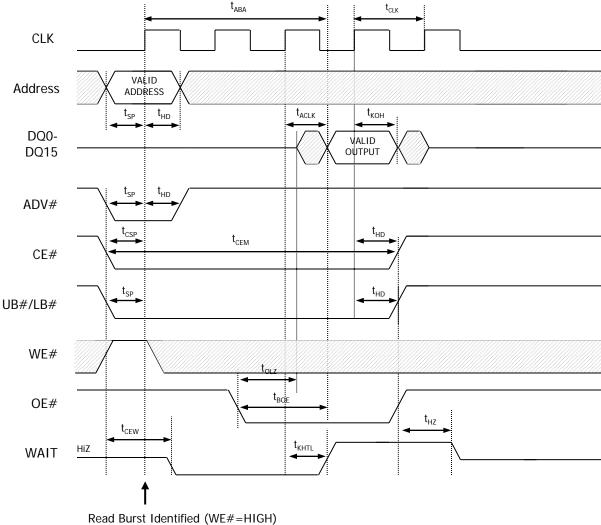
1. Non-default variable latency BCR settings for single-access burst READ operation: Latency code two (three clocks); WAIT active LOW; WAIT asserted during delay.
