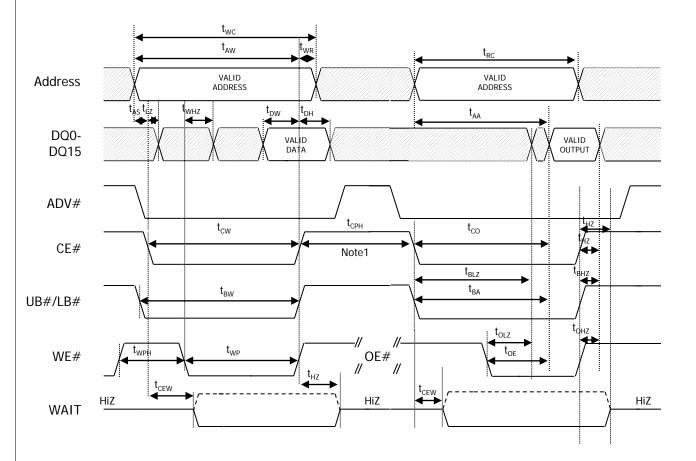
1. When configured for synchronous mode (BCR[15] = 0), CE# must remain HIGH for at least 5ns (tCPH) to schedule the appropriate refresh interval. Otherwise, tCPH is only required after CE#-controlled WRITEs.
