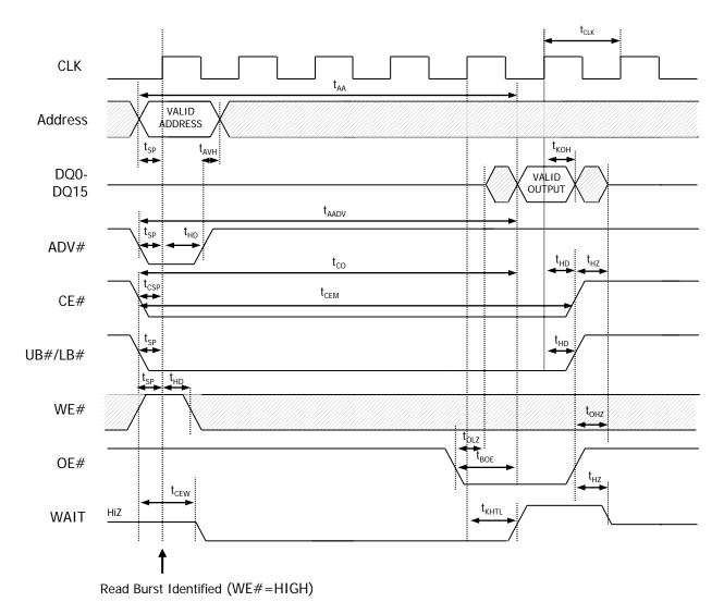
1. Non-default fixed latency BCR settings for single-access burst READ operation: Fixed Latency; Latency code four (five clocks); WAIT active LOW; WAIT asserted during delay.
