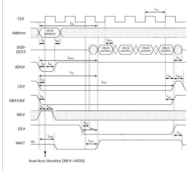
1. Non-default fixed latency BCR settings for 4-word burst READ operation: Fixed latency; latency code two (three clocks); WAIT active LOW; WAIT asserted during delay.
